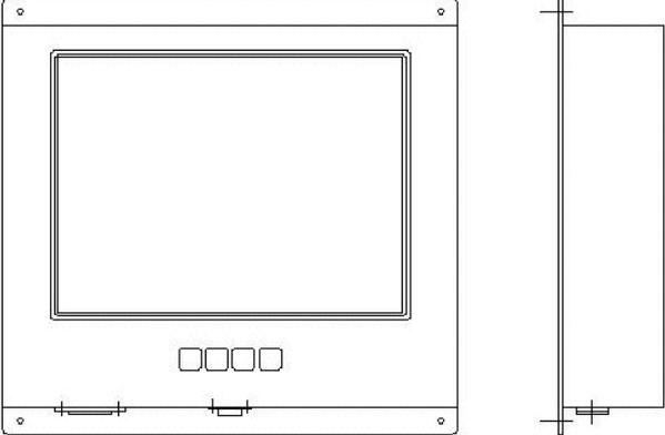
The image shows two technical drawings of the IM137 monitor. On the left is a front view showing a square monitor with a thin bezel and four mounting holes at the corners. Below the monitor, there are four small square icons representing the connector pins. On the right is a side view showing the monitor's profile, which is very thin, with a small protrusion at the bottom center.    |
